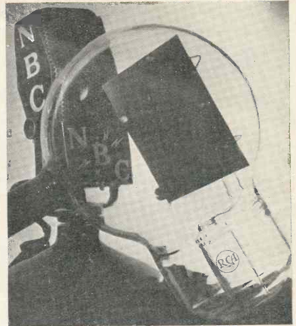
R.C.A.'s famous Iconoscope, the tube which transforms what it "sees" into electric impulses. In the background is the well-known N.B.C. microphone.
